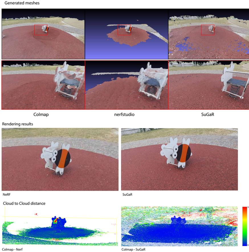
**Figure 2:** Comparison of the mesh obtained with the proposed methodologies on the playgrounds dataset. Other scenes can be found at: [https://zenos4mbu.github.io/photogrammetry\\_nerf.github.io/](https://zenos4mbu.github.io/photogrammetry_nerf.github.io/)
