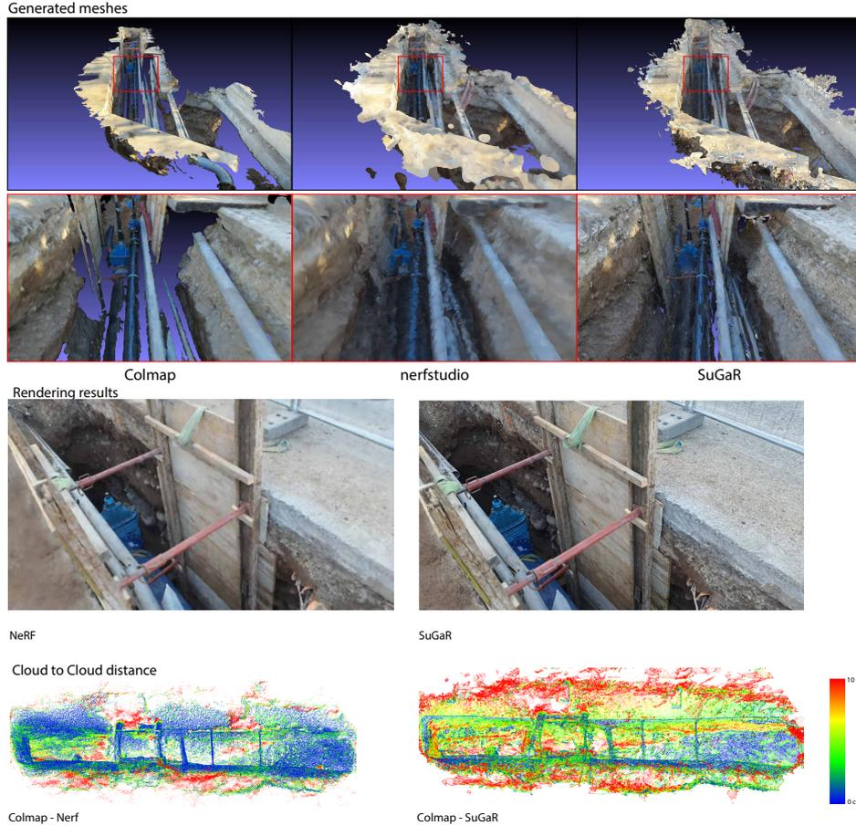
**Figure 3:** Comparison of the cloud to cloud distance of the proposed methodologies on the excavation sites dataset. Other scenes can be found at: [https://zenos4mbu.github.io/photogrammetry\\_nerf.github.io/](https://zenos4mbu.github.io/photogrammetry_nerf.github.io/)
