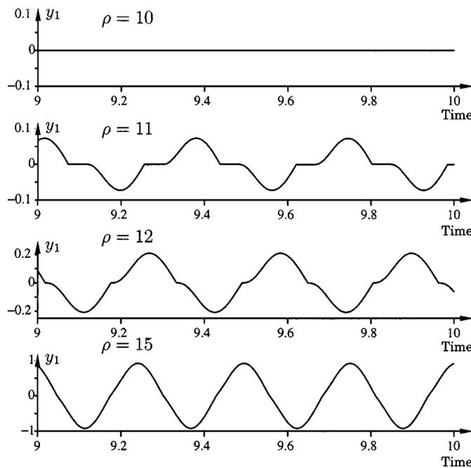
Fig. 8. Close-ups of the oscillatory behavior of the flexible servo for different values of the design parameter  $\rho$ . For  $\rho = 10$  there is no limit cycle. If  $\rho = 11$  we get a limit cycle that includes periods of sticking. For  $\rho = 12$  and 5 the velocity is zero only for single time instants.
