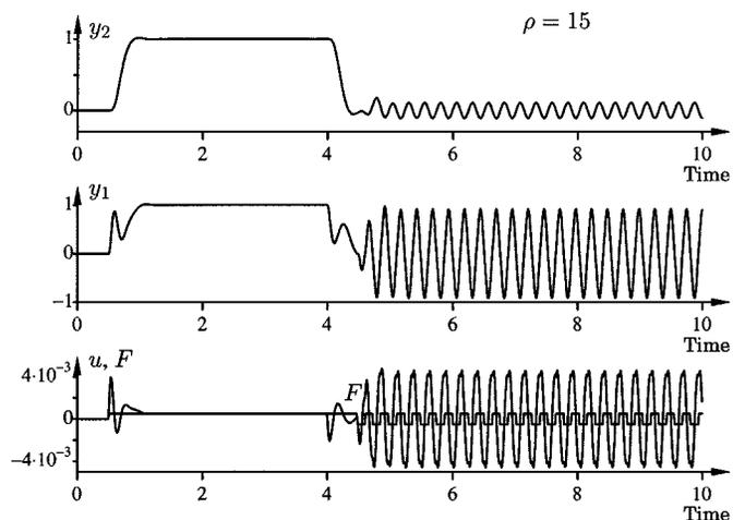
Fig. 7. Simulation of the flexible servo for  $\rho = 15$ . The limit cycle is a pure relay oscillation, i.e., the friction force switches instantly between the levels  $\pm F_C$ . The velocity  $y_1 = k_\omega \omega_1$  is almost sinusoidal.
