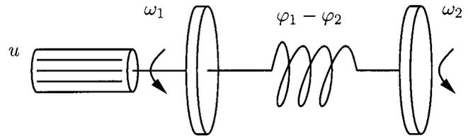
Fig. 3. A schematic picture of the flexible servo.
