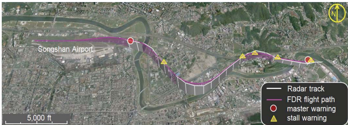
Figure 1.11-5 Superimposed GE235 GPS flight path, ATC radar track and key cockpit warnings
