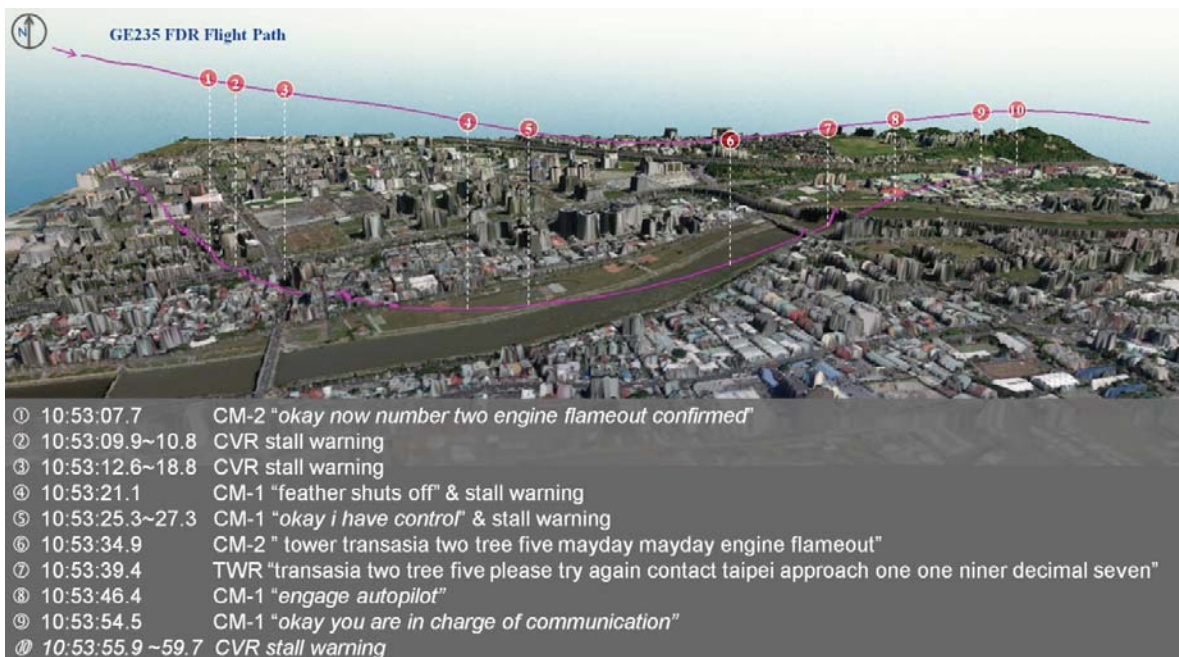
Figure 1.11-6 GE235 flight path and key events rendered on a fused satellite image and digital surface model between 1053:07.7 and 1053:59.7
