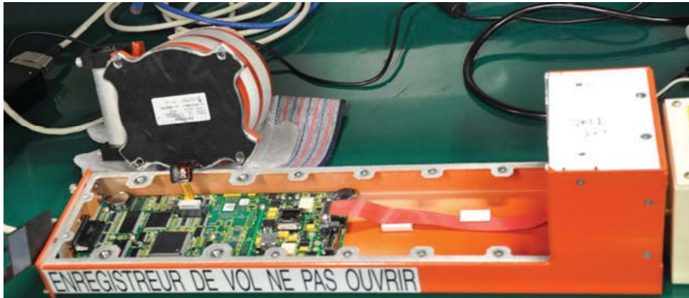
Figure1.11-3 FDR CSMU connection to chassis
