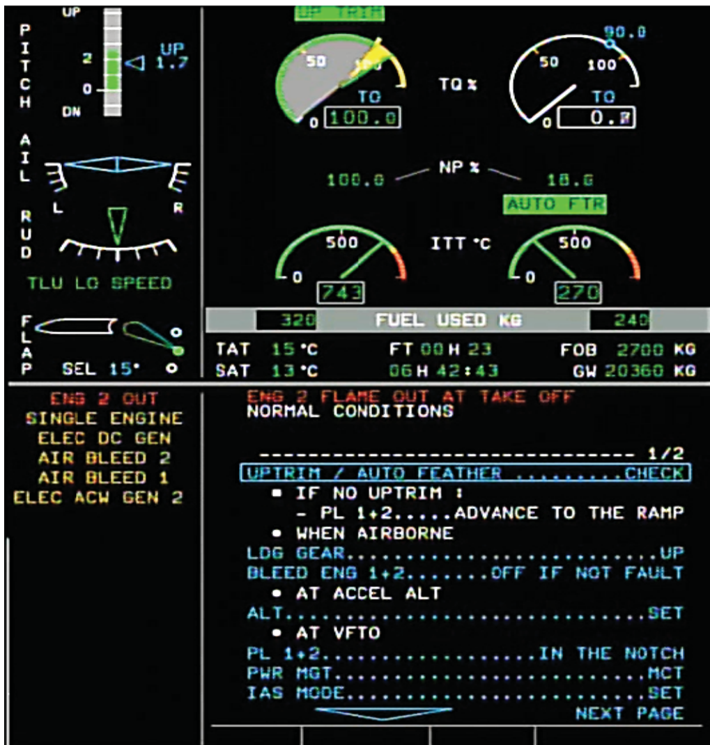
Figure 1.6-4 Simulated EWD indications for ENG 2 autofeather at take off 21
