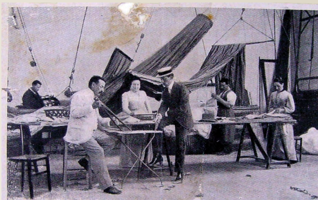
[Photograph by V. Gribayedoff, Paris.] MAKING THE NEW SANTOS-DUMONT BALLOON—WOMEN PATCHING TOGETHER THE VARIOUS SECTIONS OF THE SILK ENVELOPE IN THE WORKSHOPS OF M. HENRI LACHAMBRE, VAUGIRARD.
